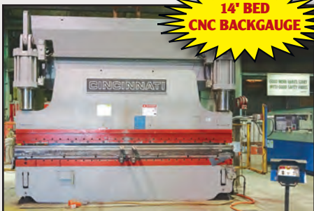
2002 CINCINNATI 350-TON CBII 14' BED, 12' BTW HOUSING, 16' STROKE, CNC BACKGAUGE
