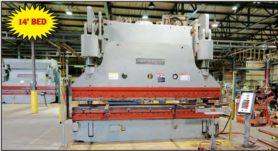
CINCINNATI 400-TON FM 14' BED, 10' BTW HOUSING, 12' STROKE, MANUAL BACKGAUGE
