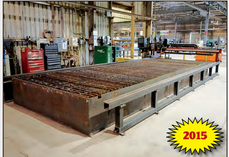
2015 THERMAL DYNAMICS ULTRA-CUT 200 XT PLASMA WITH iCNC XT 231 CONTROL ON A 8' X 24' 2006 KOIKE AROSON BRIDGE WITH (3) ADDITIONAL OXY FUEL HEADS AND BRIDGE
