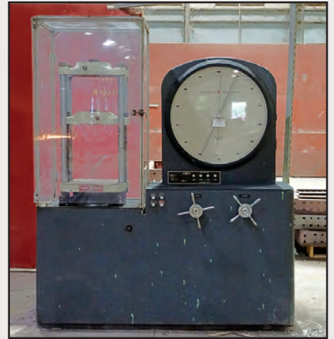
TINIUS OLSEN TENSEL TESTER MDL. SELECT RANGE
